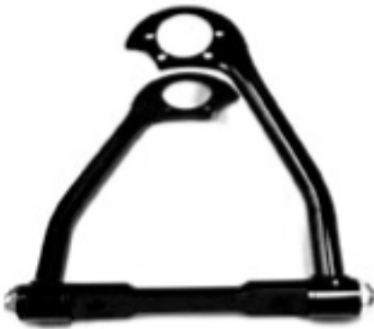
10-3/4, 11, 11 1/4 SPLIT BOLT IN UPPER LEFT
