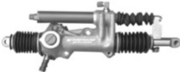
WOODWARD RACK WITH PS CYLINDER
